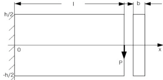
Fig.3 In-plane bending of a cantilever plate due to a boundary shear of a parabolic distribution given by
